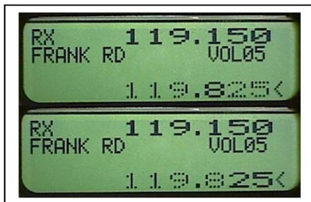
The Standby-Frequency is set with the turning knob in 3 different ranges. The selected range is highlighted and can be changed with the **FREQ** button.
