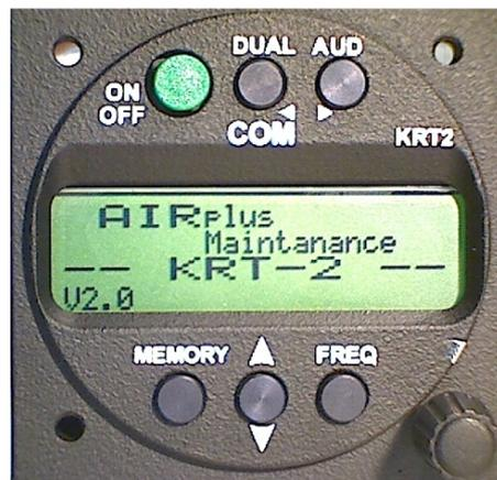
The start display shows device type and the software number. It then changes into the normal operating mode (Direct Input).
