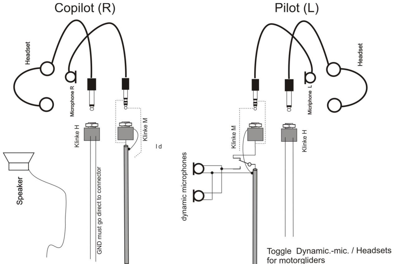
Because the 8V supply voltage is switched off when dynamic microphones are used during glider flight the second (copilot) headset microphone is disabled.
