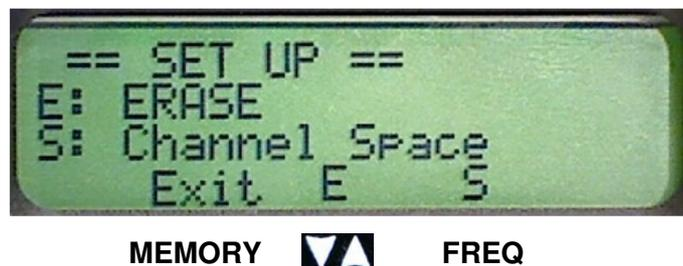
Set-up program exit is with the MEMORY button. The unit remains powered and the normal operating mode is resumed.
