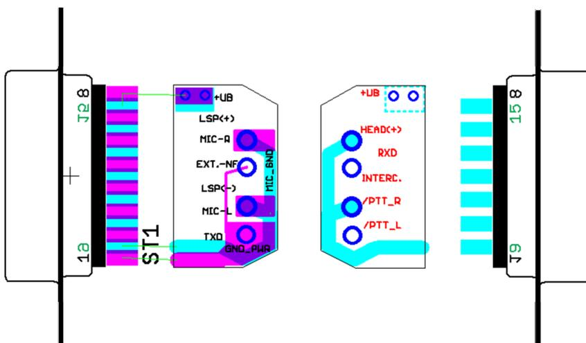
The adapter board is placed between the connector pin rows and soldered to the BAT plus pins 8,15 and GND pins 1 and frame. Pin 9 (microphone-GND) is provided on two pads for shielding. Further information printed on the board serves to connect all cables to its corresponding pins.
